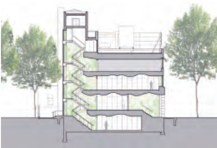
Above: A section of the Chelsea Health Center illustrates how the renovation connects the clinic to the park with a new glass-enclosed stair, undulating wood ceilings, and perimeter "park walls" Top left: Waiting rooms and circulation in the center have park views and "park walls" that evoke the surrounding sycamore trees Top right: Natural shapes and materials and high-gloss white walls in the lobby express the connection between nature, health, and the advanced care offered there
