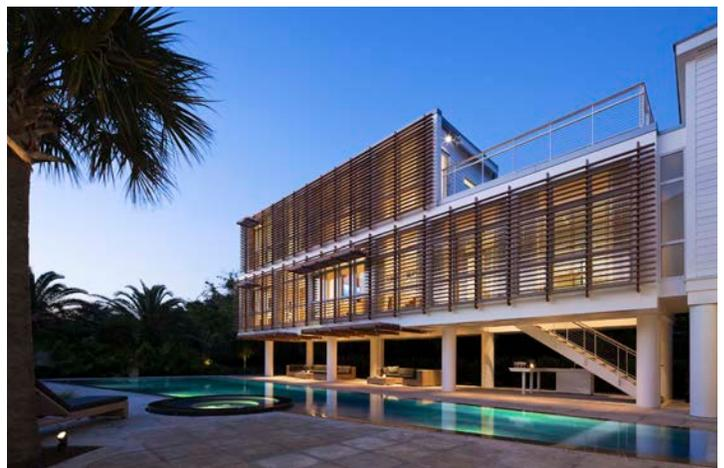
Despite being underneath a two-story guest house, the outdoor living room feels cozy rather than claustrophobic. Yablon speced steel framing for the structure so there could be longer open spans between the columns. Those columns are hefty, but the smooth, round shape harkens back to traditional low-country porches and softens the concrete-paved expanse of flooring-cum-pool decking.
